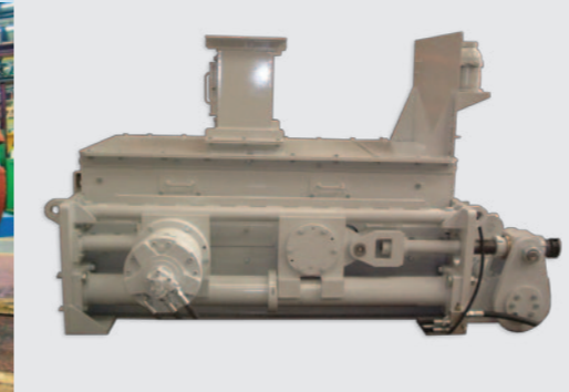
Main Right Two 3 tonne rolls in final testing for 90150 Double Roll Crusher.
